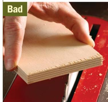
**Rough cuts.** One cause of tearout on the lower edge is a lack of support directly under the workpiece. Most of the throat plates supplied with tablesaws have a wide gap around the blade.
