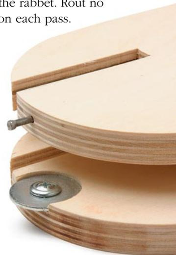
**Two types of locks.** On some saws, a fender washer fits under the throat's edge. Others need a brad or screw.
