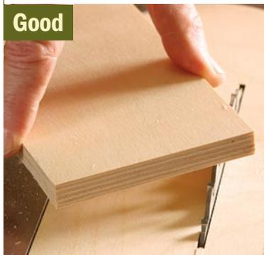
**Clean cuts.** A zero-clearance opening eliminates tearout because the workpiece is supported next to the blade.
